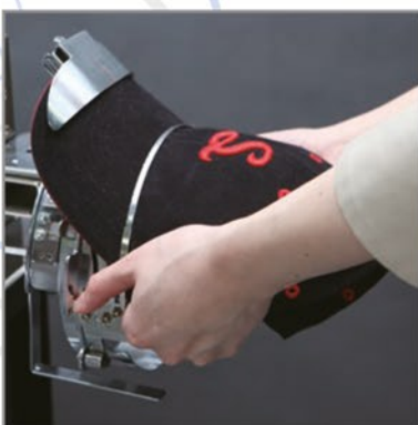
Stretch the cap over the frame
