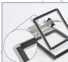
Double-sided frame surface to cover both woven and slippery material
