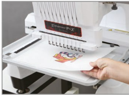
Set printed image on the frame
